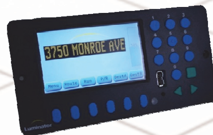
Large touchscreen can be used for information entry or programmed for advanced features.
